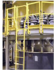
Raised platform with protected guardrail.
